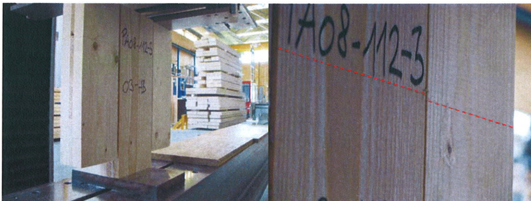
Fig. 11 Shear failure at the new developed symmetric shear block – serie ‘TUG’
