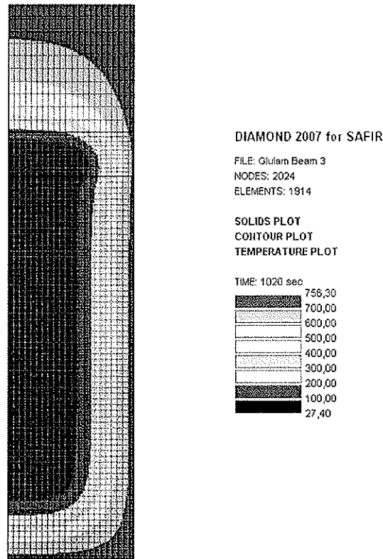
Figure 3 – Results of heat transfer analysis of unprotected beam: Temperature field after 17 minutes of fire exposure. The border of the residual cross-section is represented by the 300°C isotherm.
