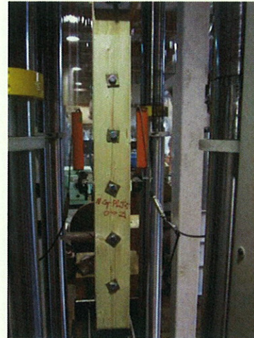
Photo.1 Lag screwed timber-to-timber joint with a pair of deflection measuring devices at middle of a fasteners.
