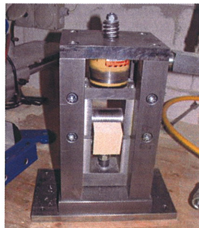
Fig. 2: Prototype of shear test equipment with a defined state of shear in the glue line
