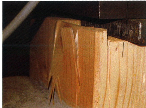
figure 5: Failure cause of series K and S - shearing of timber in front of the joint
