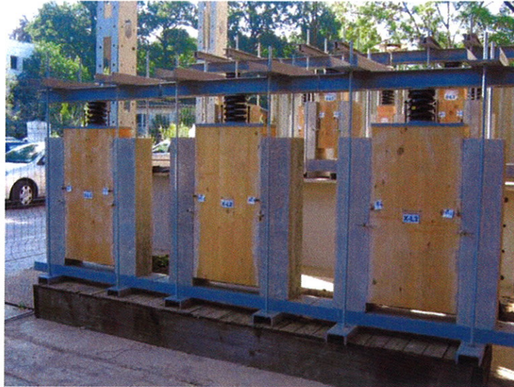
figure 9: Long-time shear tests (specimens stored outside and roofed)
