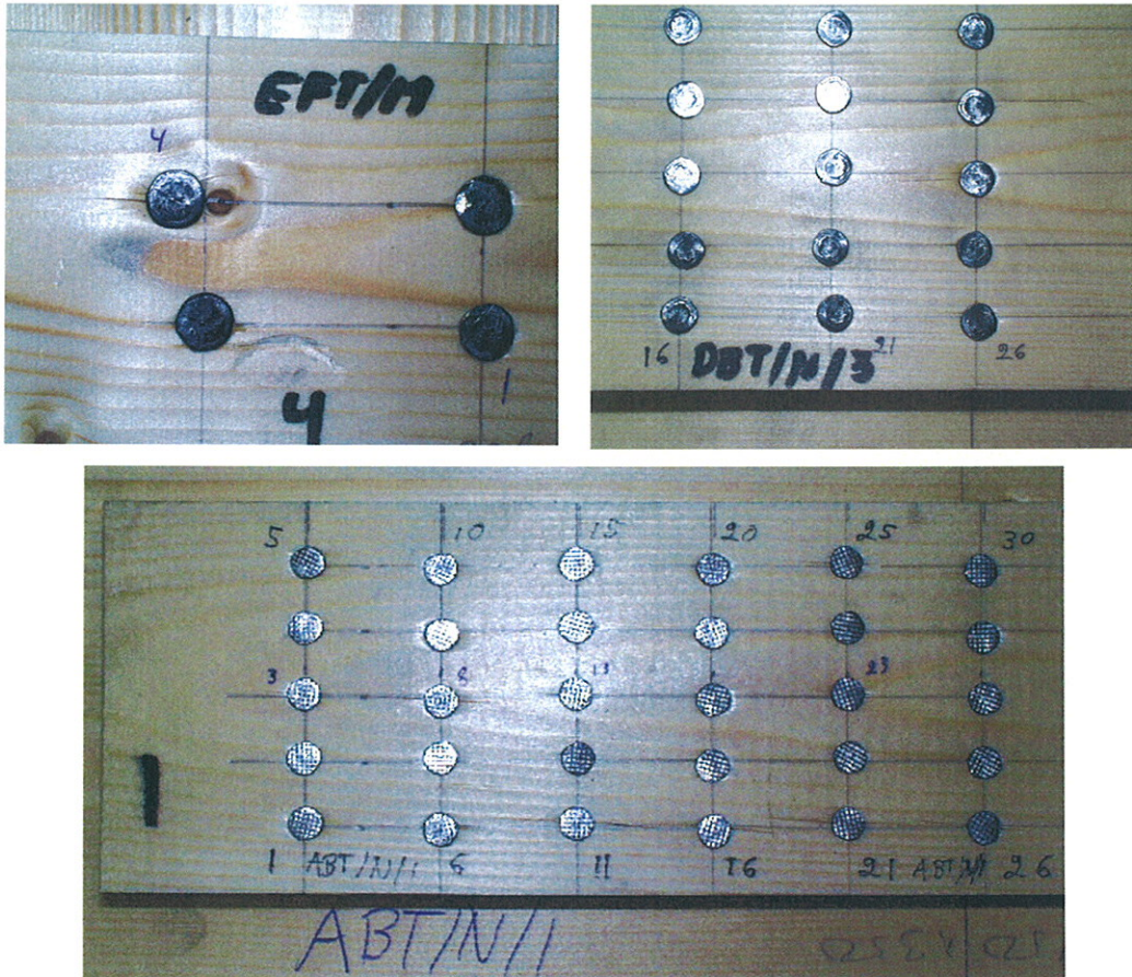
Figure 4 Examples on the biggest cracks of the nailing test specimens.
