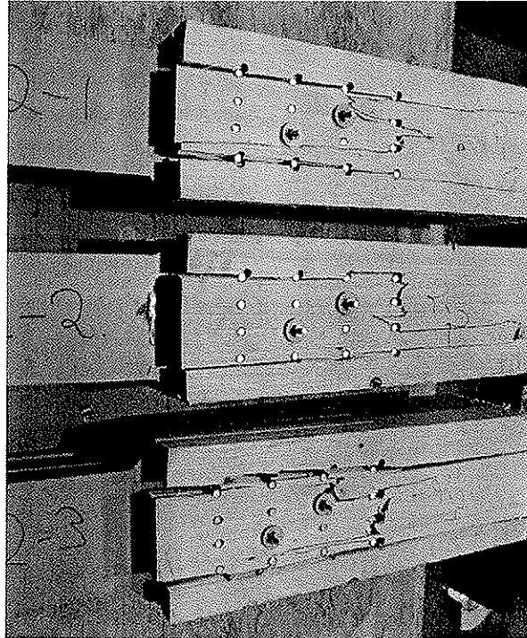
Figure 4. Dowel connections after testing.
