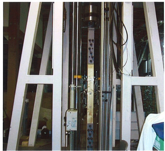
Photo.1 Servo-actuator type testing machine.
