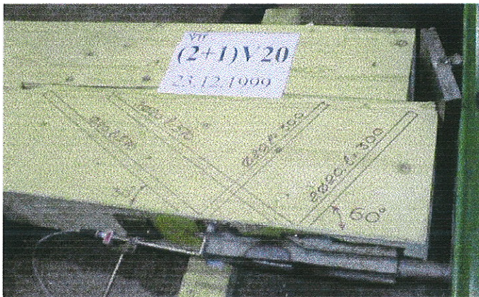
Figure 9. Shear failure at 712 kN following tensile failure perpendicular to grain.
