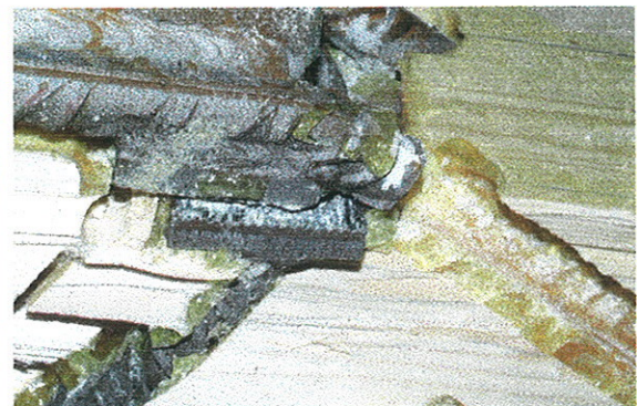
Figure 10. Test specimen 2V25 after failure at 734 kN and cut open.
