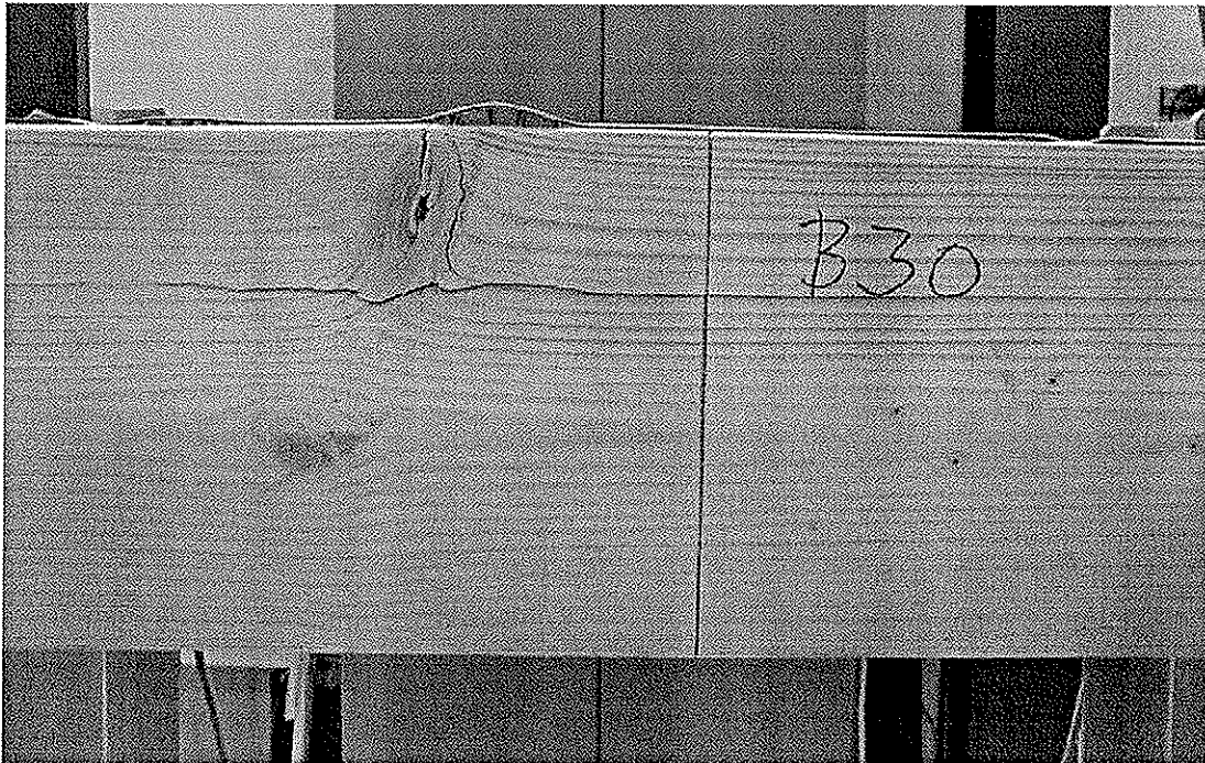
Figure 3: Extension of the plastic zone at a knot of an unloaded test in series S11.
