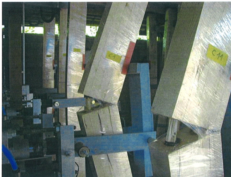
Figure 10: Failure by pull-out of rod and adhesive together
