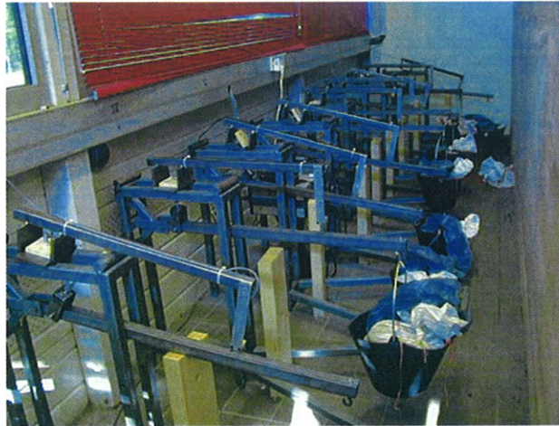
Figure 15: long term experiment set-up for small specimen
