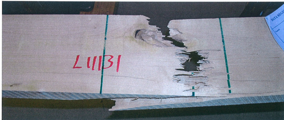
Figure 2. Tension failure at Critical Section in lamination no. L11131 (36 mm x 151 mm) Tension stress at failure: f_{t,0} = 65,7 \text{ N/mm}^2
