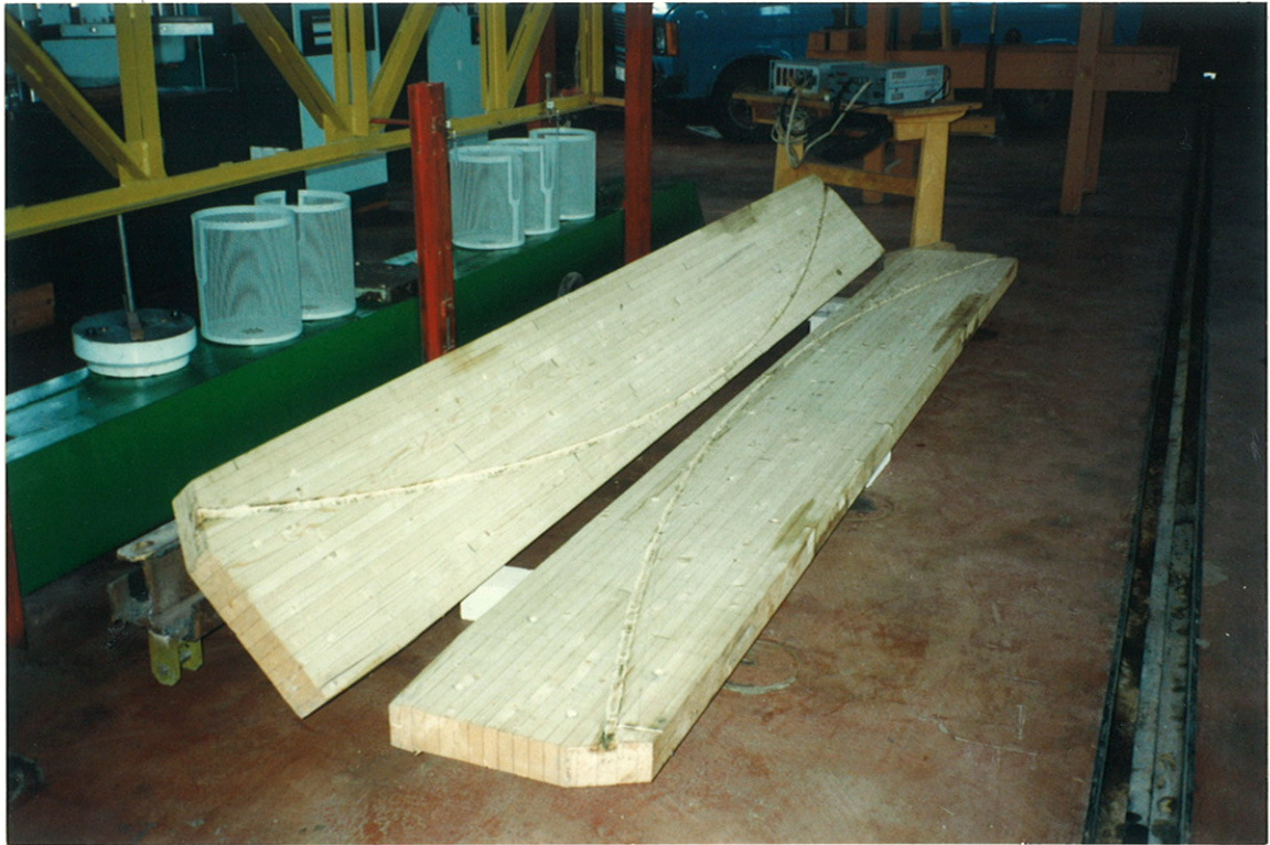
Figure 1. Halves of the tested beam with grooves for steel bars.
