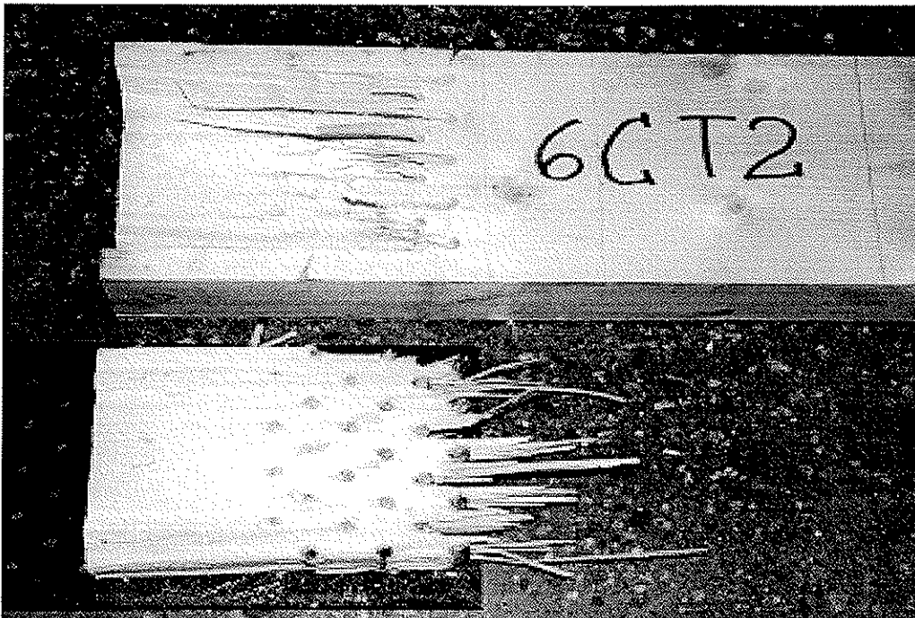
Figure 8 - Block tearing failure of test pieces made of Kerto-S-LVL (S), Kerto-Q-LVL (Q) or sawn timber (T).
