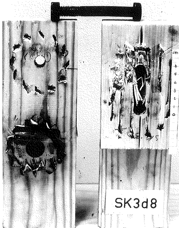
Fig. 1: Typical failure of a Bulldog tooth-plate connection
