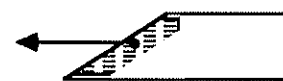
Fig. 8, If the plate plasticizes only the plate close to the joint line is active
