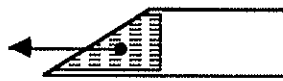
Fig. 7, If plasticity is not allowed the plate acts with its full size and the plate-timber force is located in the middle of the anchorage area
