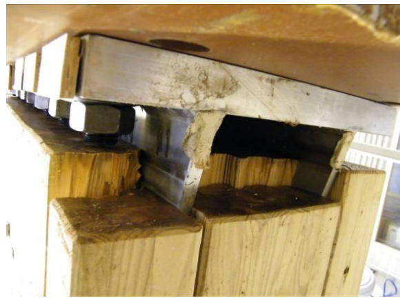
Figure 10: L block failure of rectangular grid pattern “Fondation Louis Vuitton pour la Création” connection in four-point bending loading (a) with artificial cracks on the outer parts (b) after humidification.
