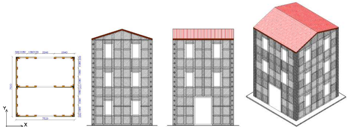
Fig. 11 Case study: modular wall panel arrangement
