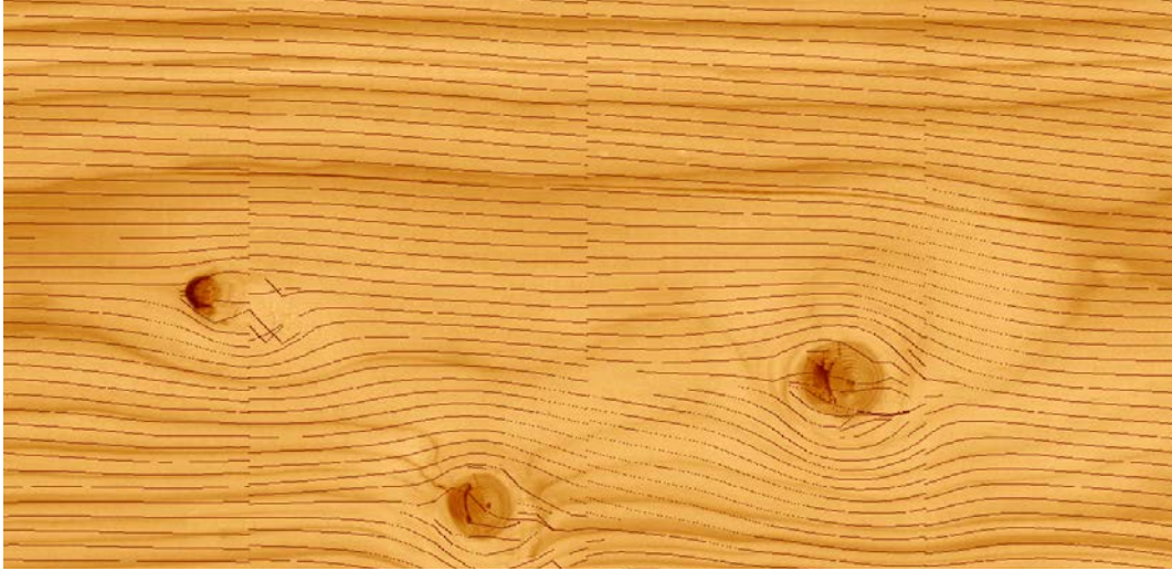
Figure 2: Fibre angle lines at outer face of a timber board obtained from laser scanning
