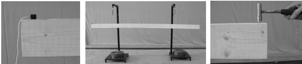
Fig. 1 A board is suspended in rubber bands (photograph in the centre). An accelerometer is fastened at one end of the board on the narrow edge (photograph to the left). In the opposite end of the board it is hit with an impulse hammer on the narrow edge (photograph to the right).
