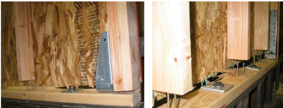
Figure 4. A combination of nail withdrawal, panel edge tear-out, and bottom plate failure from biaxial (combined shear and uplift) tests
