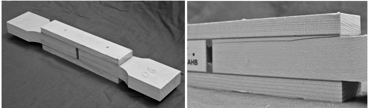
Figure 1: Adhesively bonded double lap joint: test specimen (left) and close-up at the locus of failure initiation after testing (right)
