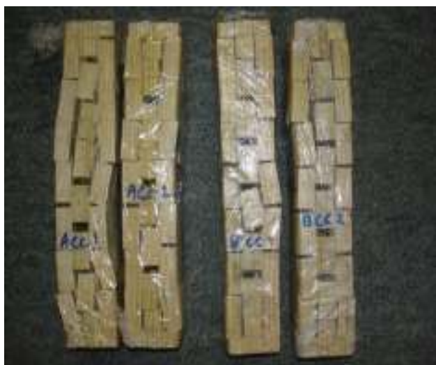
Figure 10: The API creep specimens that collapsed under 50°C conditions.
