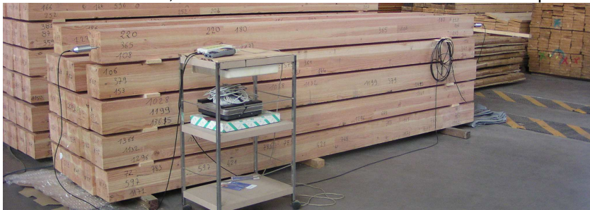
Figure 3 : NDT MOE of Glued Solid timber evaluated by UltraSonic method.
