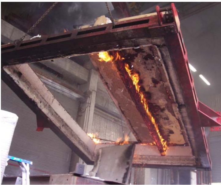
Figure 2: The Underside of the 300 mm Floor after Furnace Testing
