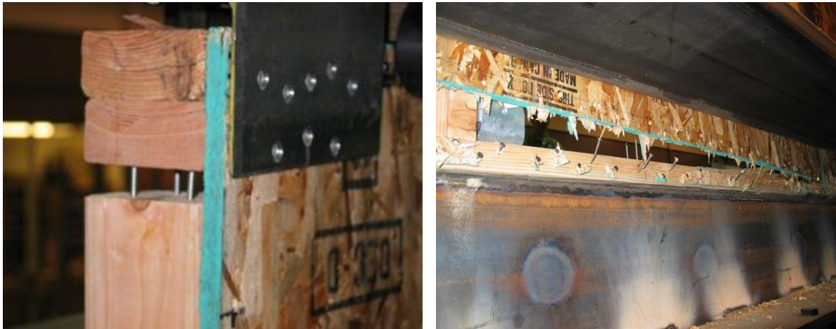
Figure 3. Nail withdrawal from bottom and top plates, and panel edge tear-out from uniaxial (uplift-only) tests
