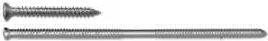
Figure 2. Top: Self-drilling spun screw. Bottom: SFS- screw with thread both under the head and at the end, (the pitches are a little different resulting in the parts being drawn tight together).
